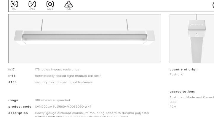
powder coat finish and impact-resistant GRP security caps Impact-resistant UV-stabilised high-transmission polycarbonate light module diffuser Serviceable replaceable and upgradable light module cassette Internal socket drive security-torx 304 stainless steel security fasteners Integral energy efficient Zhaga compliant Tridonic LED modules and power supply unit Heavy-gauge stainless steel wire suspensions
