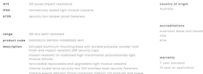
Integral energy efficient Zhaga compliant Tridonic LED modules and power supply unit Direct-fix or recessed butterfly bracket Internal stainless steel wire safety lanyards 1.0 m circular flex connection
