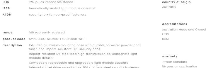
Internal socket drive security-torx 304 stainless steel security fasteners Integral energy efficient Zhaga compliant Tridonic LED modules and power supply unit Direct-fix or recessed butterfly bracket Internal stainless steel wire safety lanyards
